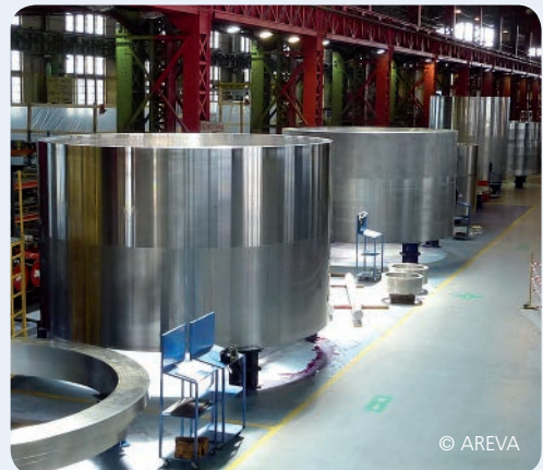
End of machining for steam generator shell
