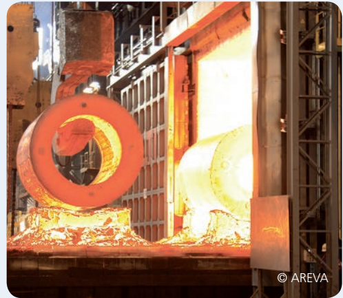
Pre-heating of steam generator shell
